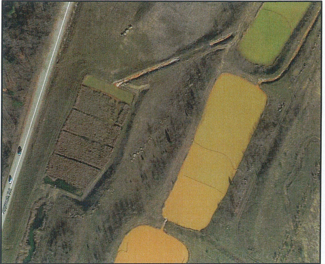
Photo showing the effectiveness of polishing wetland at removing suspended iron to below detection on Hach testing kit.
